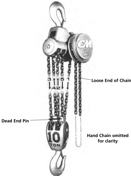
FIGURE 21. Reeving 10 Ton Hoists
