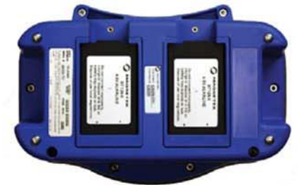
Main battery and spare battery packs
