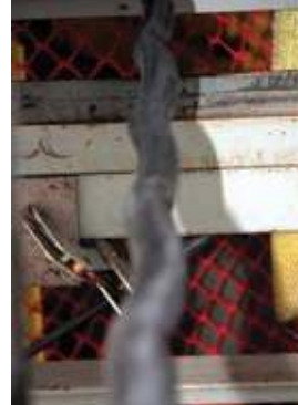
Failing cable due to the “corkscrew” effect
