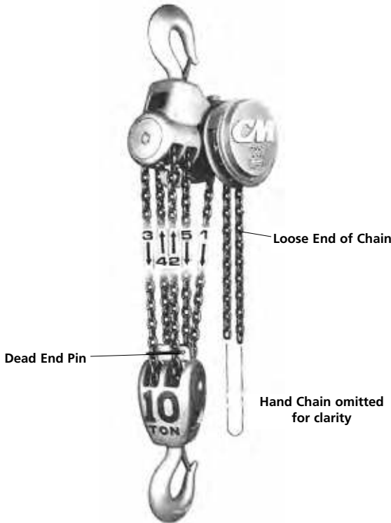
FIGURE 21. Reeving 10 Ton Hoists
