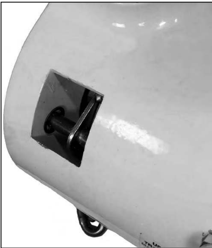
Figure 7-13. Removing Chain Guide Support Pins
