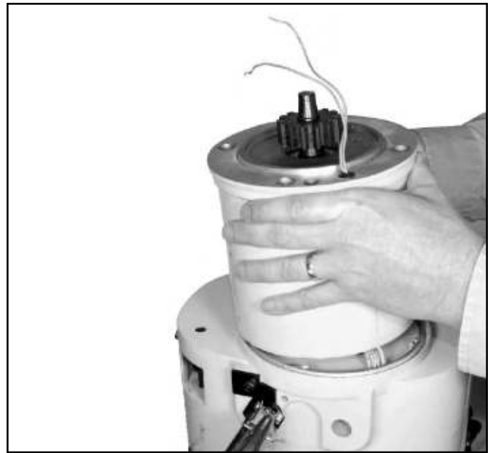
Figure 7-9. Removing Motor Assembly
