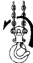
Figure 3 - Correcting Chain Twist
