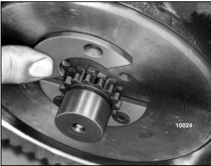
Figure 5-5. Installing Retainer Plates on Load Brake Shaft
