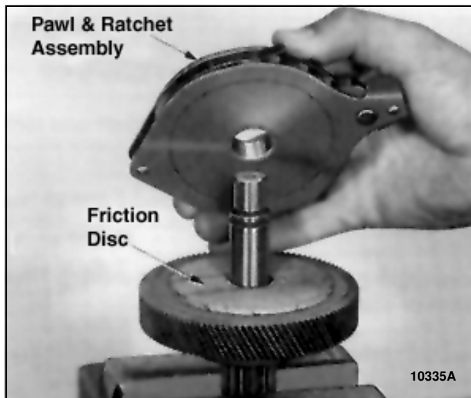
Figure 5-8. Removing Pawl and Ratchet Assembly From Load Brake Shaft
