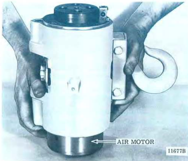
Figure 7-7. Removing Motor from Frame.
