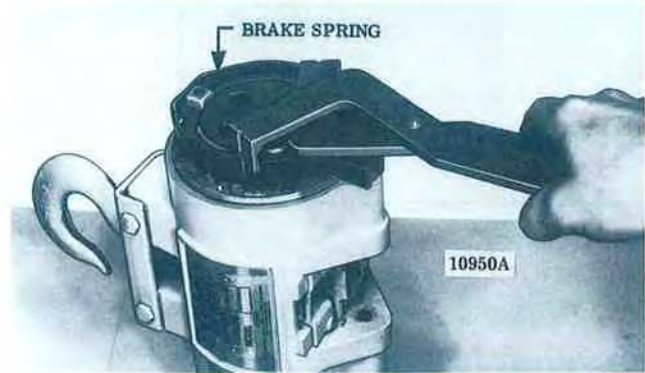
Figure 7-5. Removing Brake Spring Using Special Tool.
