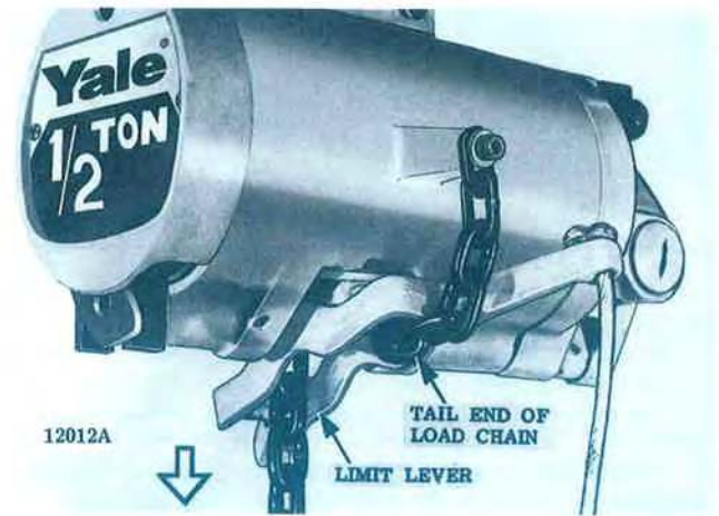
Figure 3-4. Control Lever Being Tripped by Tail End of Load Chain.
