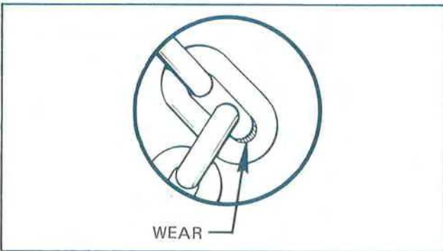
Figure 5-1. Check Chain Wear at Bearing Surfaces Between Links.
