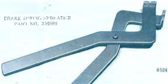
Figure 7-4. Special Tool for Removing Brake Spring.
